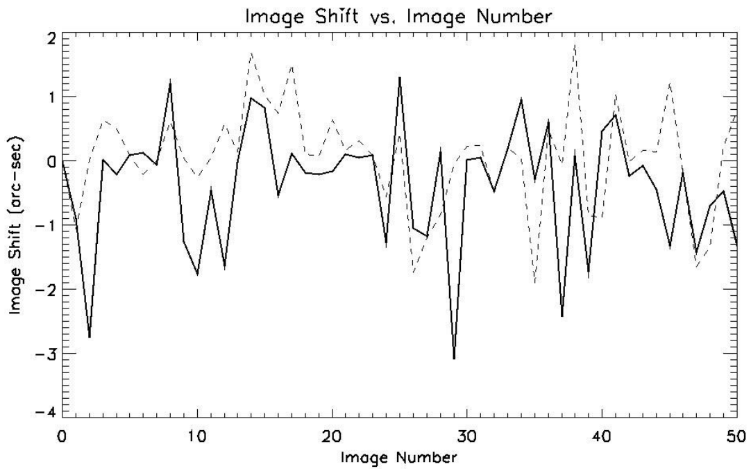
Figure 3.24 Plot of image translation of a set of magnetograms in arc-sec vs. image number.
