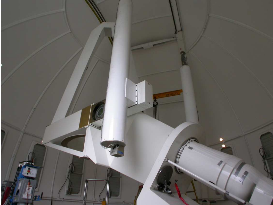
Figure 2: The NST equatorial mount, mirror cell, counterweights (for right ascension balance), and tower to secondary.
